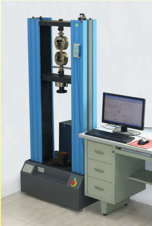
Tensile strength and elongation at break equipment
